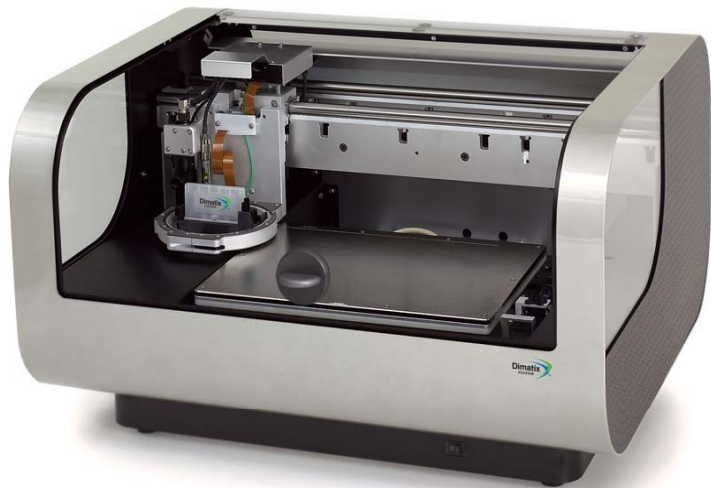
Printer used in electrode fabrication
