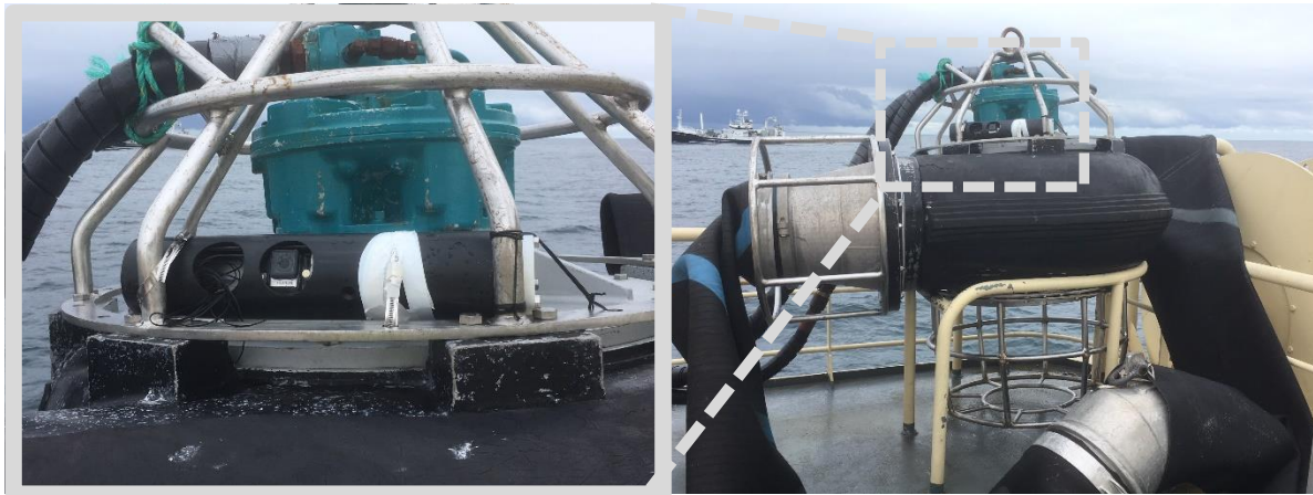
Figure 4.1. The Catch Monitoring Probe fitted to the catch pump.
