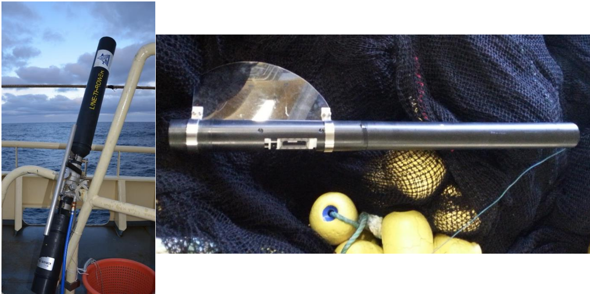
Figure 5.1: Catch monitoring probe (CMP) in protective housing (right) prepared for deployment from a compressed air canon (left).
