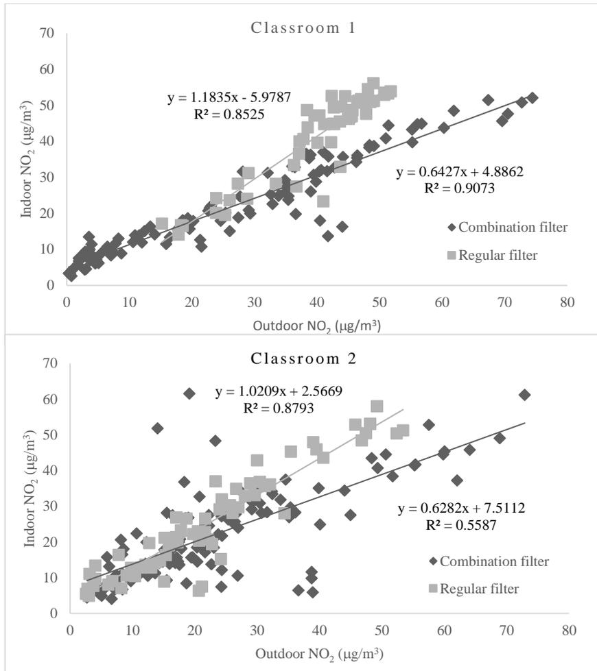
**Fig. 4.** Scatterplots of 1-h average (00-24 hours) NO<sub>2</sub> concentrations measured outdoor and indoor during sampling period 3-4 (upper) and 5-6 (lower).
