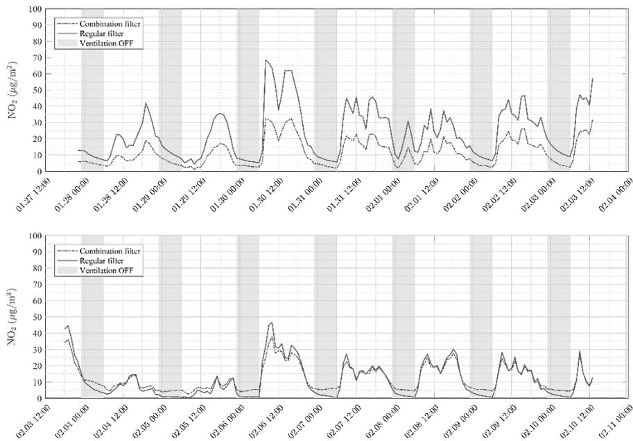
**Fig. 3.** NO<sub>2</sub> concentrations measured simultaneously inside two classrooms during sampling period 1 and 2. The filters in the ventilation systems of the two classrooms were switched between the measurement periods. Values are 1-h averages.
