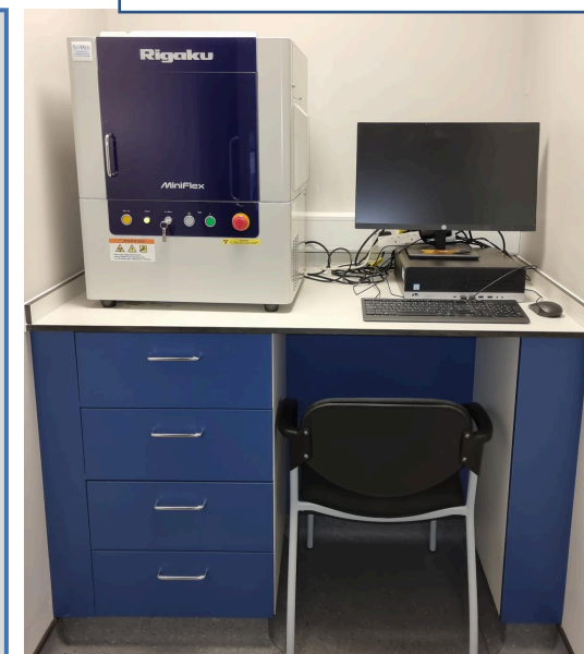
XRD to monitor bath chemistry
