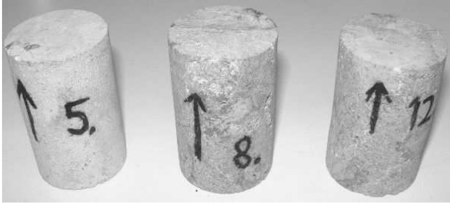
Fig. 2.9. Three core plugs with diameter of one and a half inches, and a height of five centimeters.
