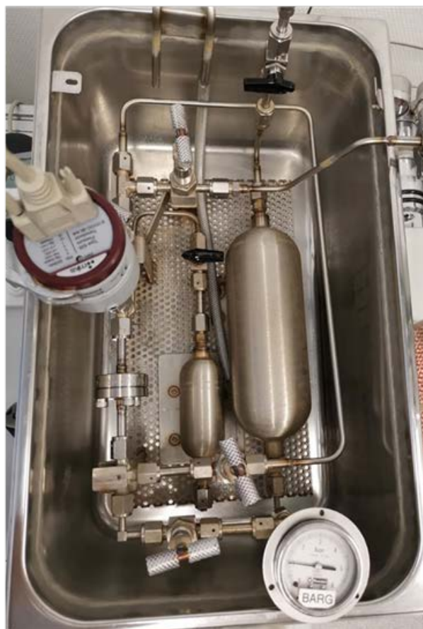
Figure 2. Gas permeation equipment to measure the CO 2 transport properties up to 25 bars, in the temperature range of 5 to 70 °C.
