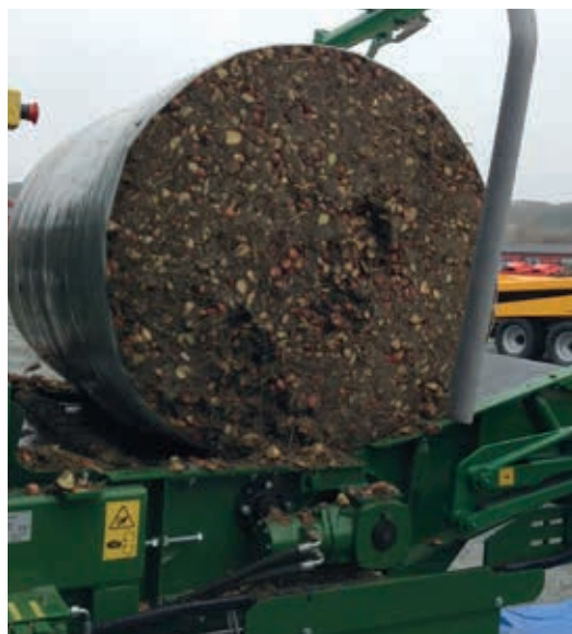
Potatoes were ensiled in a round bale, using an Orkel compactor MP2000.
