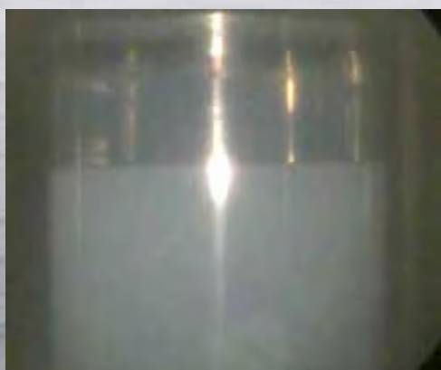
Approaching critical point in a CO 2 /N 2 mixture
