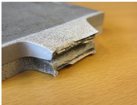
Illustration of shear fracture surfaces in small-scale steel test specimens. (Source: SINTEF)
