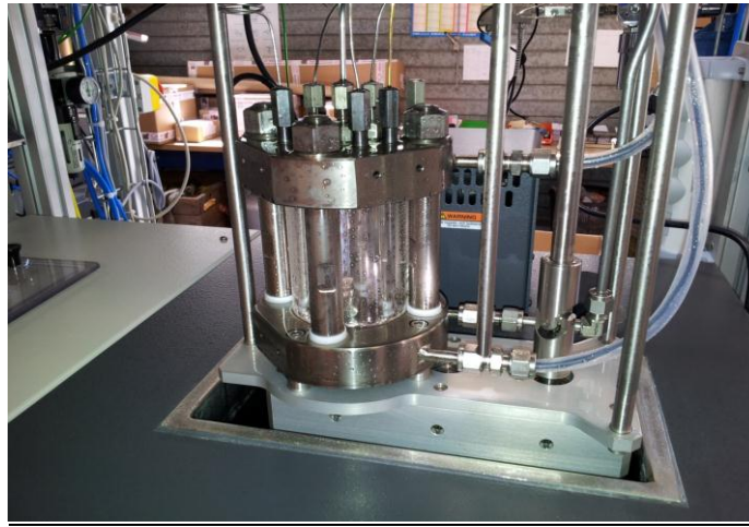
Test cell for measurement gas-liquid composition of CO 2 -rich mixtures at equilibrium. (Source: SINTEF)
