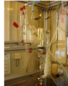
Figure 1. 1 – ebulliometer; 2 – pressure controller; 3 – temperature controllers; 4 – cold trap; 5 – buffer vessel; 6 – vacuum pump with a buffer vessel
