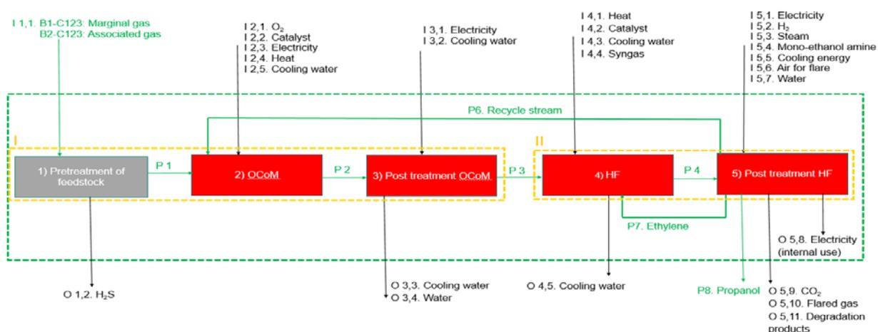
Figure 9: Simplified process design of C123 Scenarios B1 and B2. The red boxes represent the five major steps to produce propanol. The inputs (I) and outputs (O) are also mentioned. The box for the pretreatment of the feedstocks is coloured grey, because this step is not included at this moment. This pretreatment will be considered in the future dependent on the detailed composition of the feedstocks.
