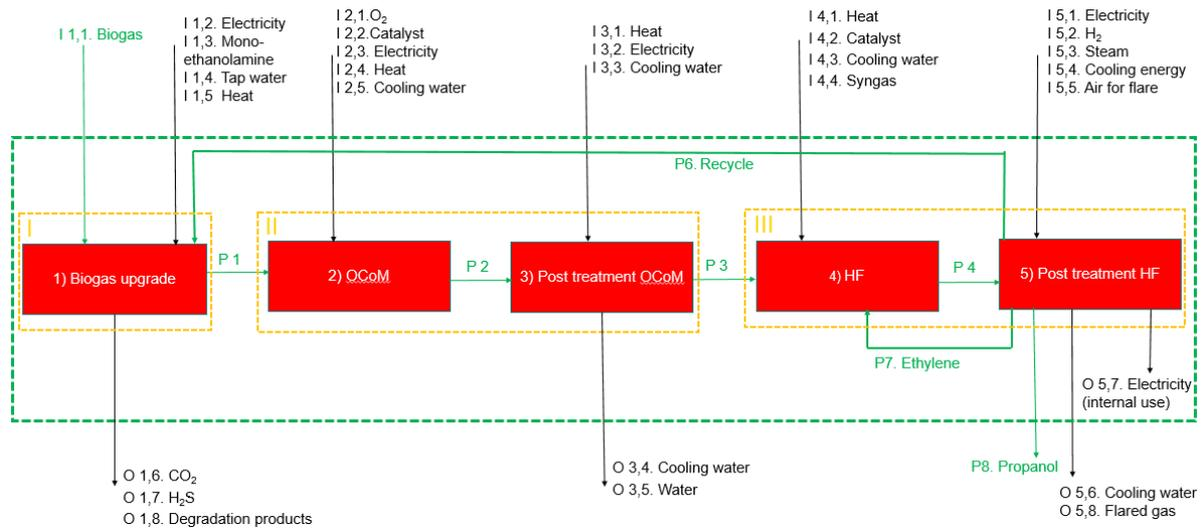
**Figure 8: Simplified process design of C123 Scenario A used for LCA analysis. The red boxes represent the five major steps to produce propanol. The inputs (I) and outputs (O) are also mentioned.**
