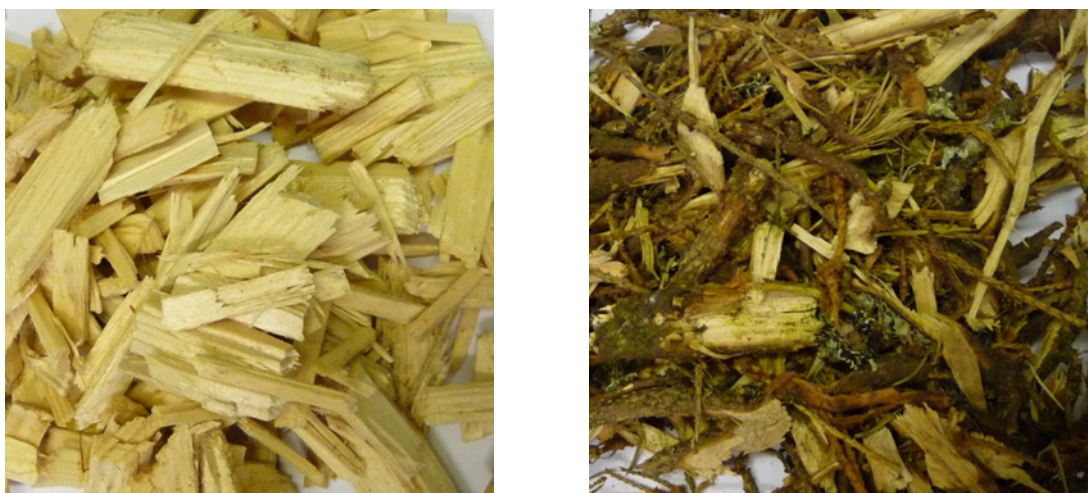
Figure 11: Different biomass qualities in Norway; wood chips (left) and branches (right) (photo: Eirik Nordhagen)
