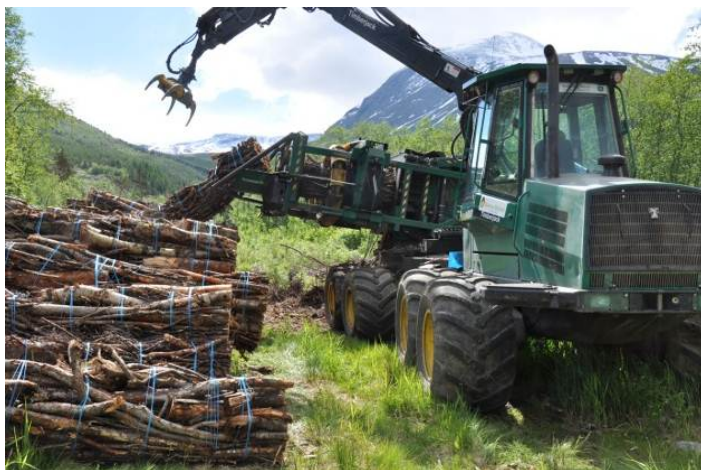
Figure 8: John Deere bundler in action (photo: Leif Kjöstelsen)
