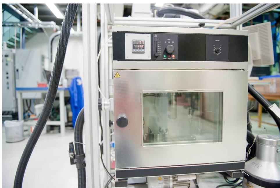
Figure 30: FTIR gas sampling and conditioning unit (photo: Sascha Njaa, SINTEF)
