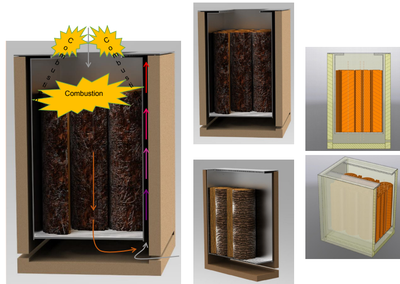
Figure 28: New wood log gasification concept adaptable for fireplaces.
