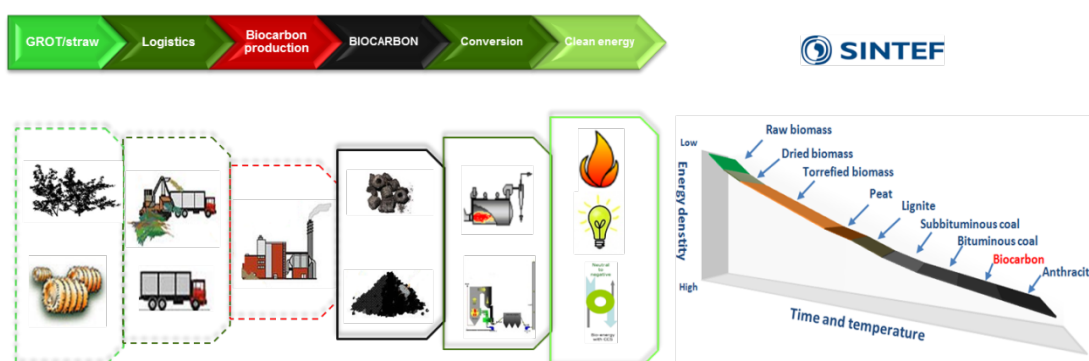
Figure 21: The BC value chain and BC energy density compared to other fuels.
