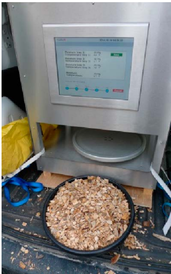
Figure 11: The moisture meter and chips in the bucket. Ready for measurements. Photo: Eirik Nordhagen
