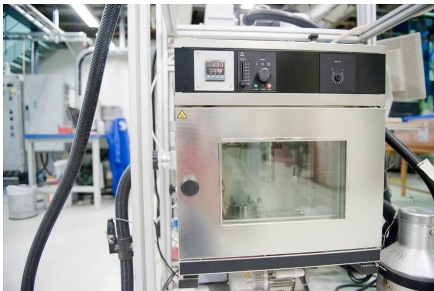
Figure 23: FTIR gas sampling and conditioning unit. (Photo: Sascha Njaa, SINTEF)
