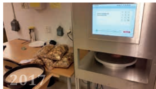
NIR Prediktor Spektron measuring moisture content of wood chips in real time. Photo: Eirik Nordhagen.
