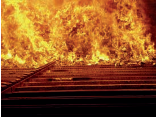
Ongoing start of waste combustion in one of Statkraft Varme's grate combustion chambers.
