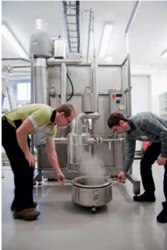
Lab-scale steam explosion unit for processing woody biomass prior to feeding into a biogas reactor. Featuring NMBU professor Svein Jarle Horn (right) and NMBU research scientist Bjørge Westereng (left). Photo: Odd Jarle Skjelhaugen.
