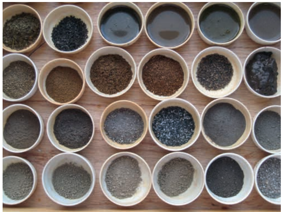
Phosphorus-rich waste materials used as fertilizer in a pot experiment.
