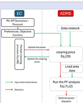
*The conceptual model to integrate the multi-EC with flexible loads in the distribution system.*
