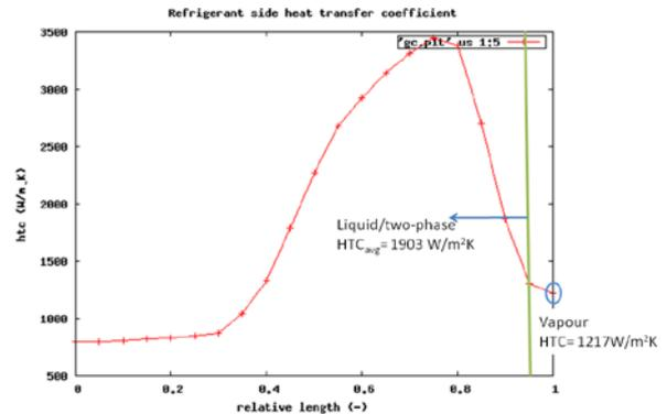
Figure 3: Heat transfer coefficient through an evaporator.
