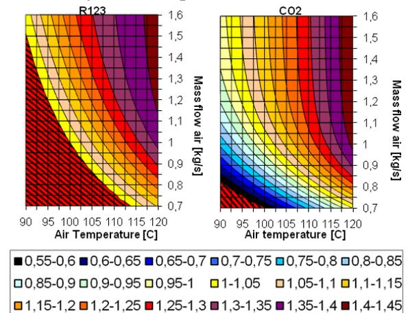
**Figure 4:** Simulation results from the two cycles when the volume flow through the expander is kept constant. The black cross indicates the design point.
