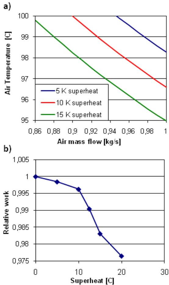
**Figure 5:** Superheating, a) critical operation line, b) reduction in work at design point.
