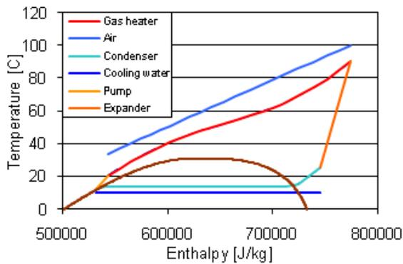
Figure 2: T-h chart, CO<sub>2</sub> cycle
