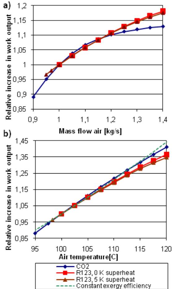
**Figure 6:** Relative reduction in work output with: a) constant heat source temperature (100 °C), b) constant a mass flow (1 kg/s).
