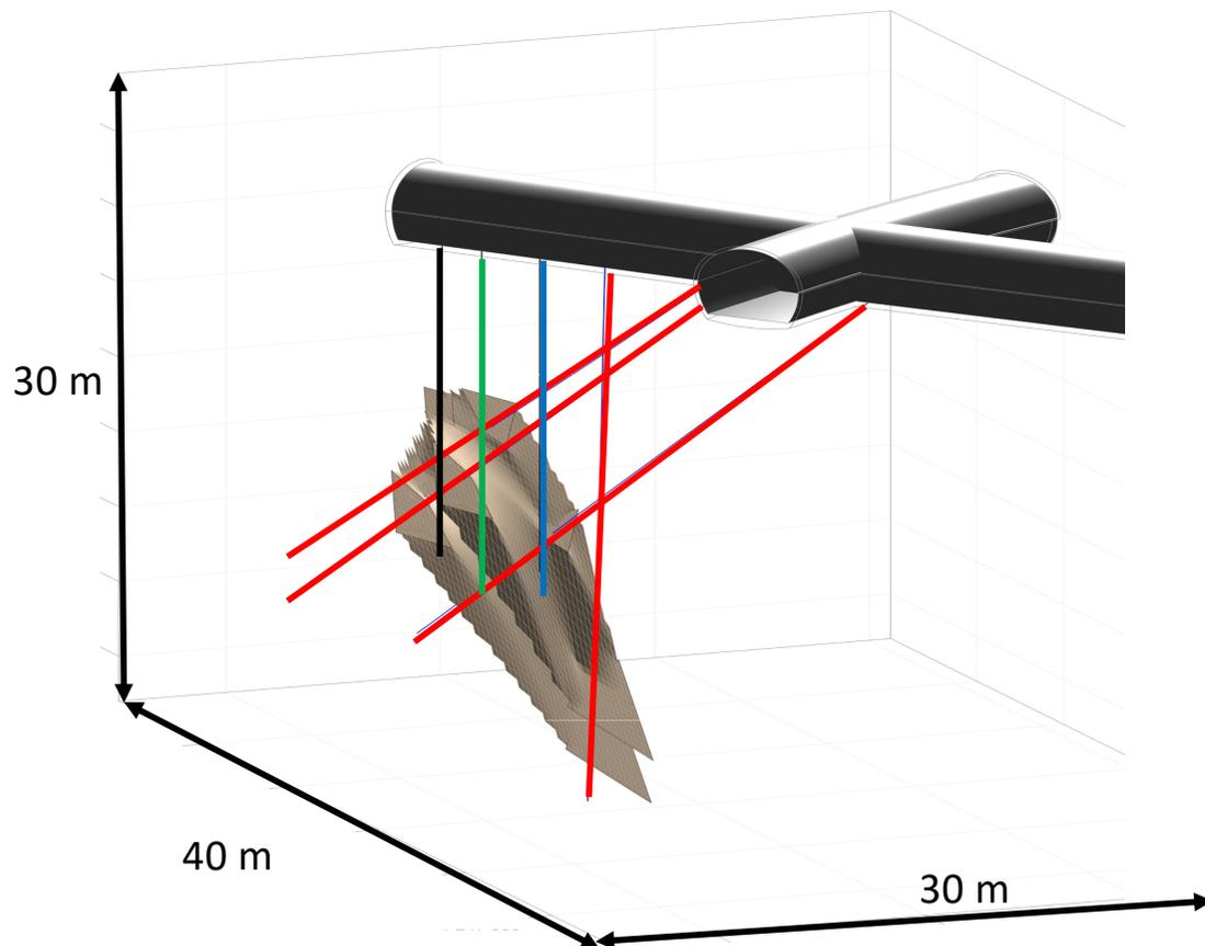
4 Boreholes for **geophysical monitoring**
