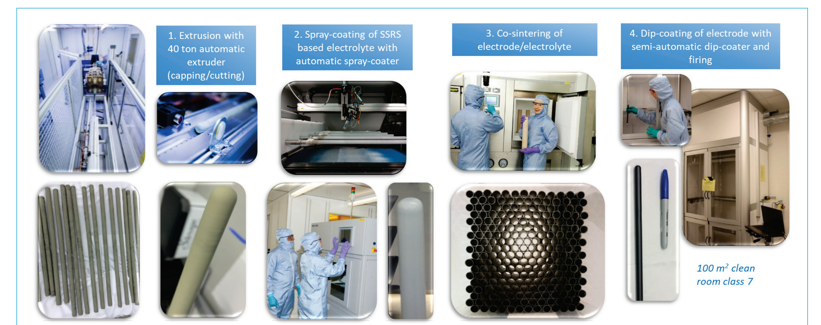
Figure 6: Manufacturing line for the production of tubular cells uses proven scaleable processes
