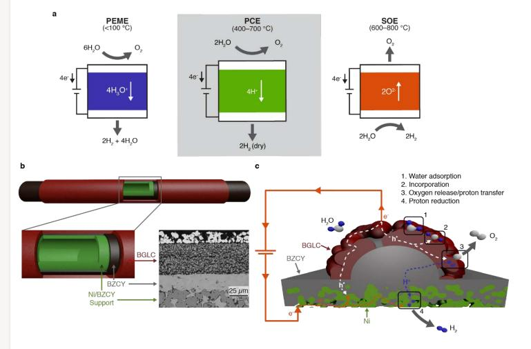
BGLC is selected as steam anode to promote mixed protonic electronic conduction and facilitate water splitting reaction
