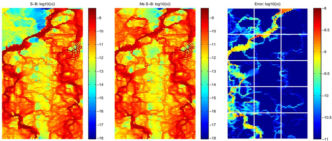
**Figure 3** Velocity magnitude computed using the fine scale Stokes–Brinkman equations (left column), multiscale Stokes–Brinkman (middle column) and velocity discrepancy overlaid by coarse grid (right column).
