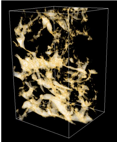
**Figure 2** Volume rendering of the 3D channels connecting the top and bottom of the model. Gray color shows the voids volumes and the void borders are shown in a yellowish color. To simplify the visualization, we have filtered out all isolated void spaces that are completely surrounded by the porous matrix, so that the figure only shows the vugs that are connected to the top and bottom of the sample.
