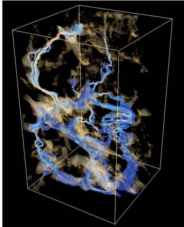
**Figure 5** Stokes flow inside the fractures and vugs, without considering the porous matrix. Blue color of the streamlines denotes low velocity, red color marks high velocity. The model has 800 000 cells and eight million nodes.
