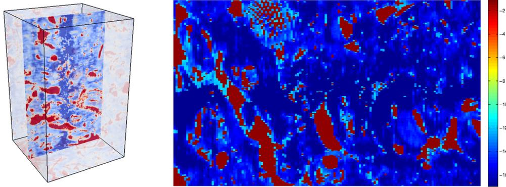
**Figure 1** Permeability of for the 3D model given on a regular grid with  $240 \times 240 \times 144$  cells. The left plot shows the 3D permeability with a 2D cut through the domain. Here, red color denotes the void spaces (vugs). The right plot shows a 2D cut with permeability plotted on a logarithmic scale.
