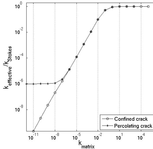
**Figure 4** Comparison of the effective permeability of a through-going and a confined fracture in a square domain with a fracture of diameter  $\ell = 0.01$ .
