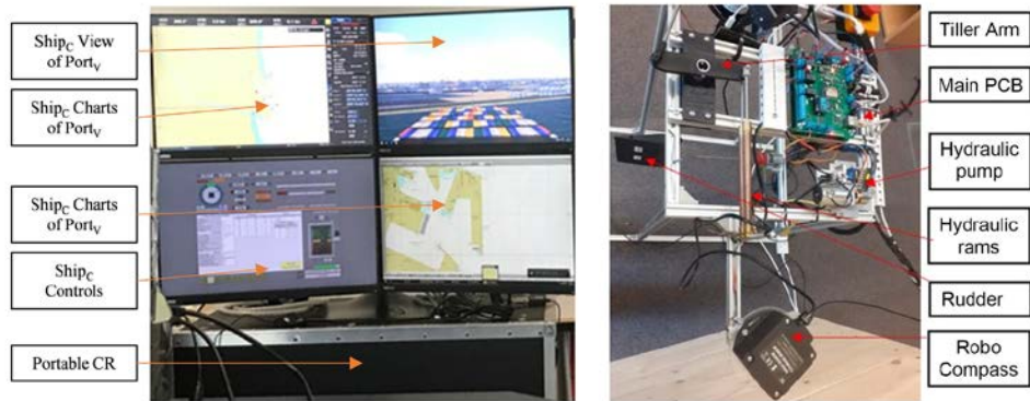
Figure 4. CR displays on top of portable CR computers and servers on left, main rudder testbed components on right with some systems like ECDIS out of view for security purposes, and the “attacker’s” computer.
