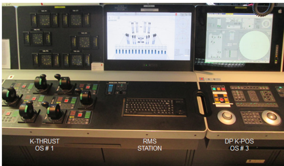
Figure 2: Close up of manual lever desk, riser management desk, and one DP desk. The utility panel is top left on the riser management desk
