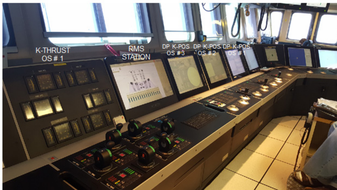
Figure 1: Bridge View showing manual lever control desk, RMS riser management desk, and three DP control desks.
