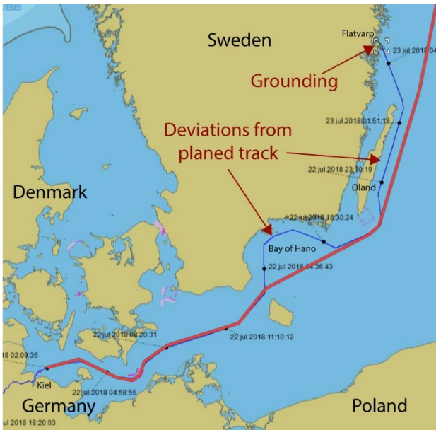
Figure 3: The red line is the planned and validated route plan for MAKASSAR HIGHWAY's voyage between Kiel, Germany, towards Sodertalje, Sweden. The blue line is the actual AIS track sailed. Times here are in UTC, i.e. Swedish summer time +2H. Adapted from [1].
