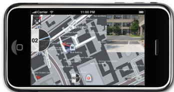
Map Display and General Interface of MAV-VUE for high level control
