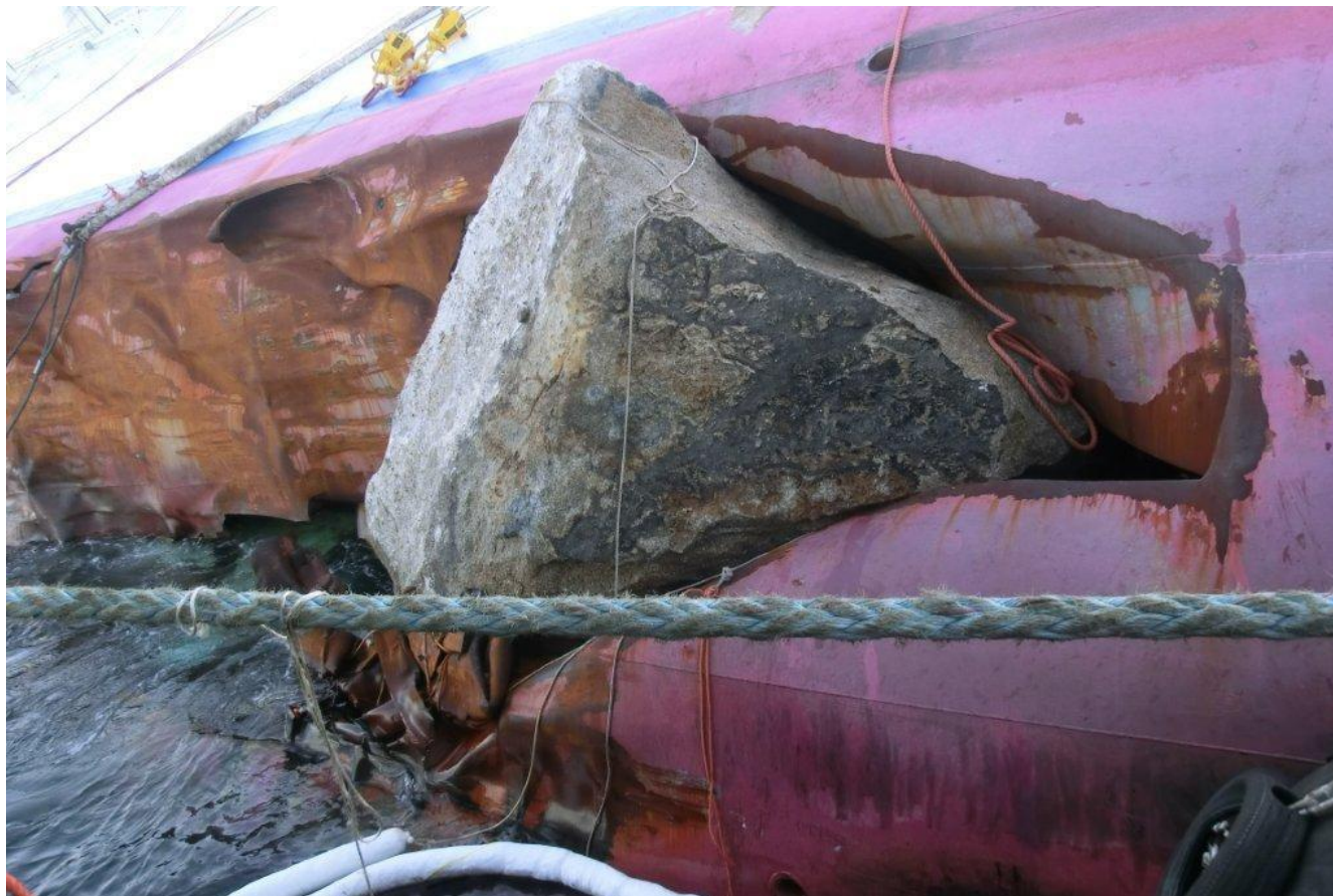
Detached rock in damaged area
