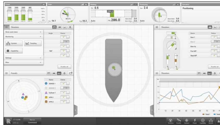
Dynamic positioning system, 24" screen
