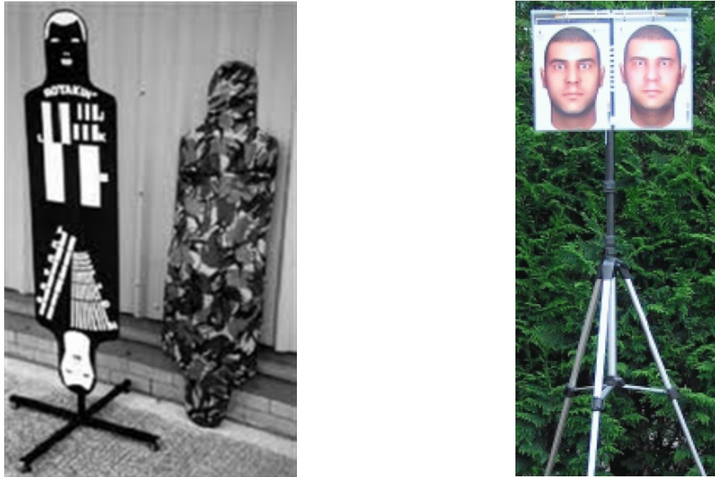
Figure 6. Rotakin (left) and additional facial test charts.
