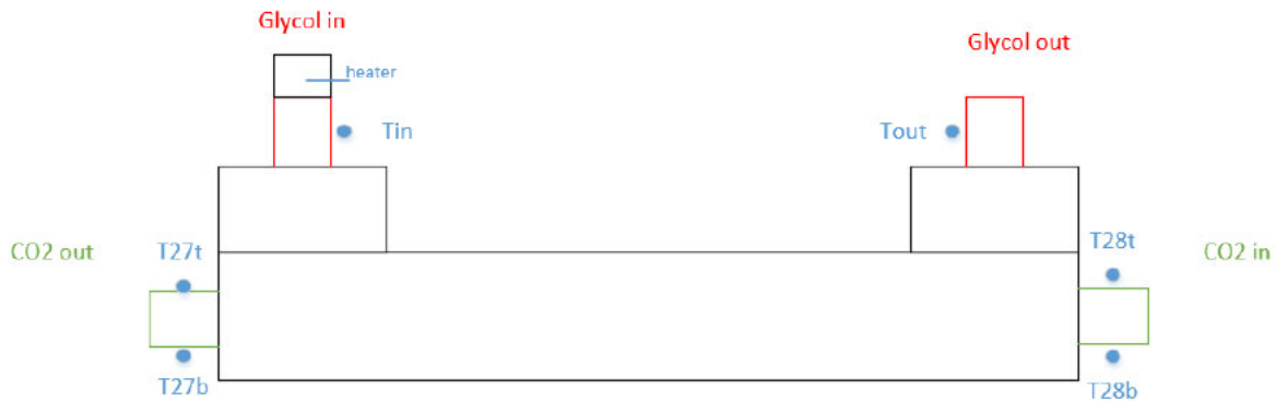
Fig. 5 Temperature sensors at the heat exchanger (evaporator)
