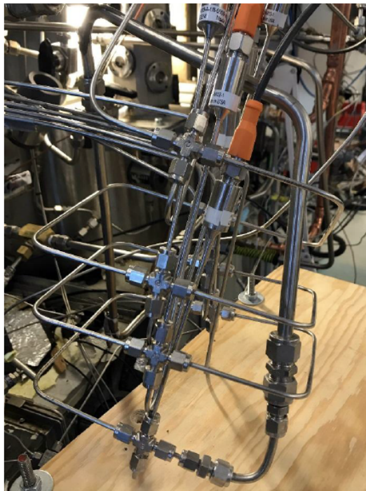
Figure 3: Capillary tube installed in the test rig.
