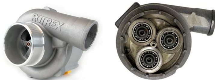
Figure 12: Compact Turbo-Compressor with lubricated planetary gearbox, up to 100 000 rpm, 200 kW thermal , impeller diameter smaller 100mm.
