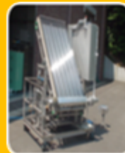
Solar water heater using supercritical CO 2
