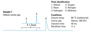
Analysis of permanent gases on a 10 m Molesieve 5Å column.
