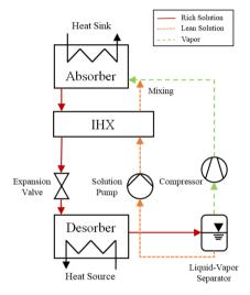
ammonia and water as natural working fluid. Heat is extracted and released at non-constant temperature glides and the required compression ratio is lower compared to conventional vapor compression heat pumps. These properties make the CACHP system interesting for the use in various industrial high temperature applications up to 150 °C.
