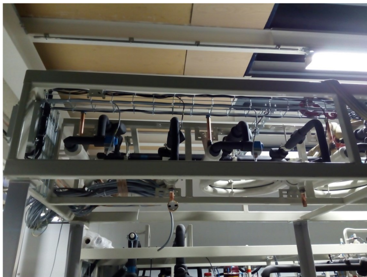
Top left, AC multiejector block (provided by Danfoss AS). Bottom left, compressor pack as delivered by Advansor AS. Above, glycol-heated evaporators to emulate the load profile of a medium size supermarket.
