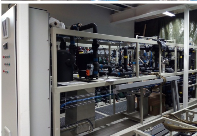
Top left, AC multiejector block (provided by Danfoss AS). Bottom left, compressor pack as delivered by Advansor AS. Above, glycol-heated evaporators to emulate the load profile of a medium size supermarket.
