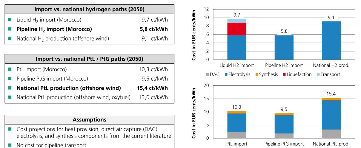
Offshore wind LCOE equal 5 ct/kWh
