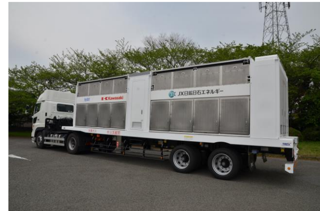
Compressed H2 trailer trucks
