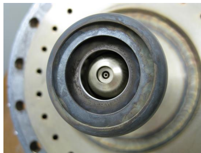
The nozzle after test
