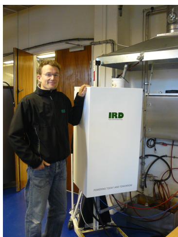
Fig. 3 Key numbers and pictures (almost the same scale) of IRDs hydrogen fuelled \mu CHP based on the LT PEM technology.
