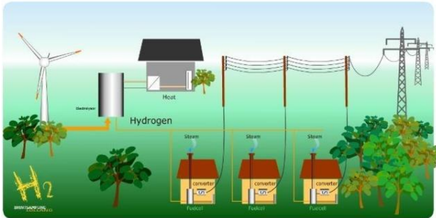
Figure 2 Field test at Vestenskov, Denmark, at which in total 32 PEMFC based CHP systems have been deployed in households, from which real life data has been fed into the KeePEMalive project for comparison to accelerated stress tests.
