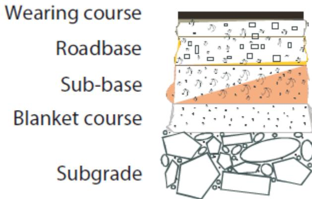
Figure 20: Typical road structure.
