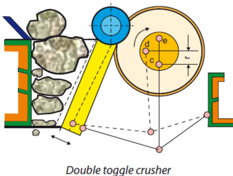
Figure 7: Double toggle crusher.
