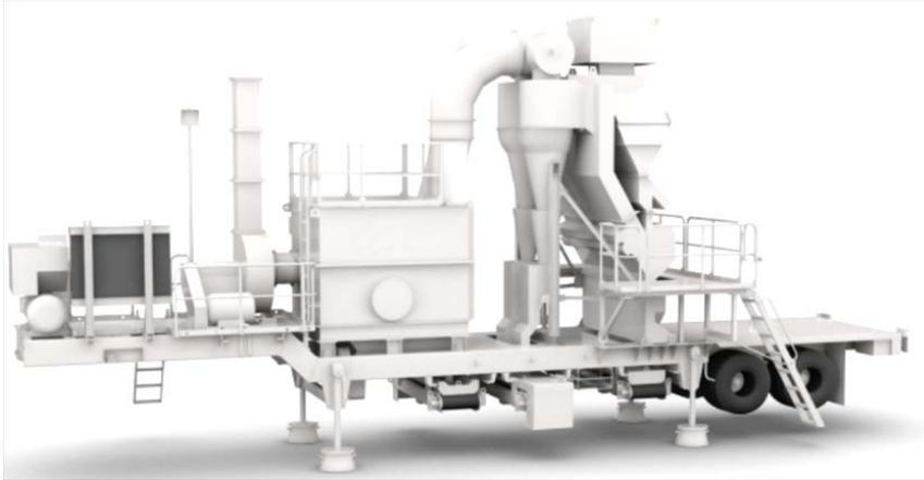
Figure 31: Metso portable static air classifier for ultra-fines removal.
