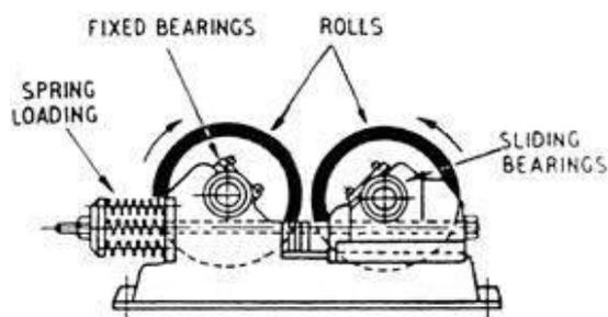
Figure 13: Traditional low-pressure roll crusher.
