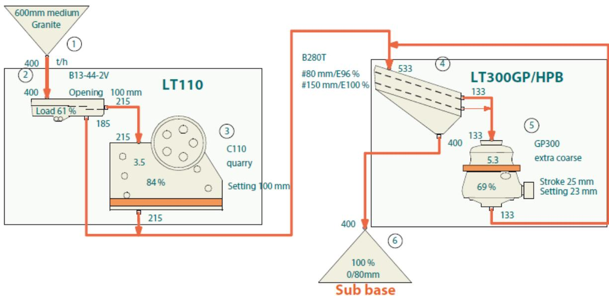
Figure 21: Typical subbase production flowsheet.
