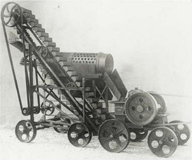
Figure 18: Mobile crushing and screening plant from the early days.
