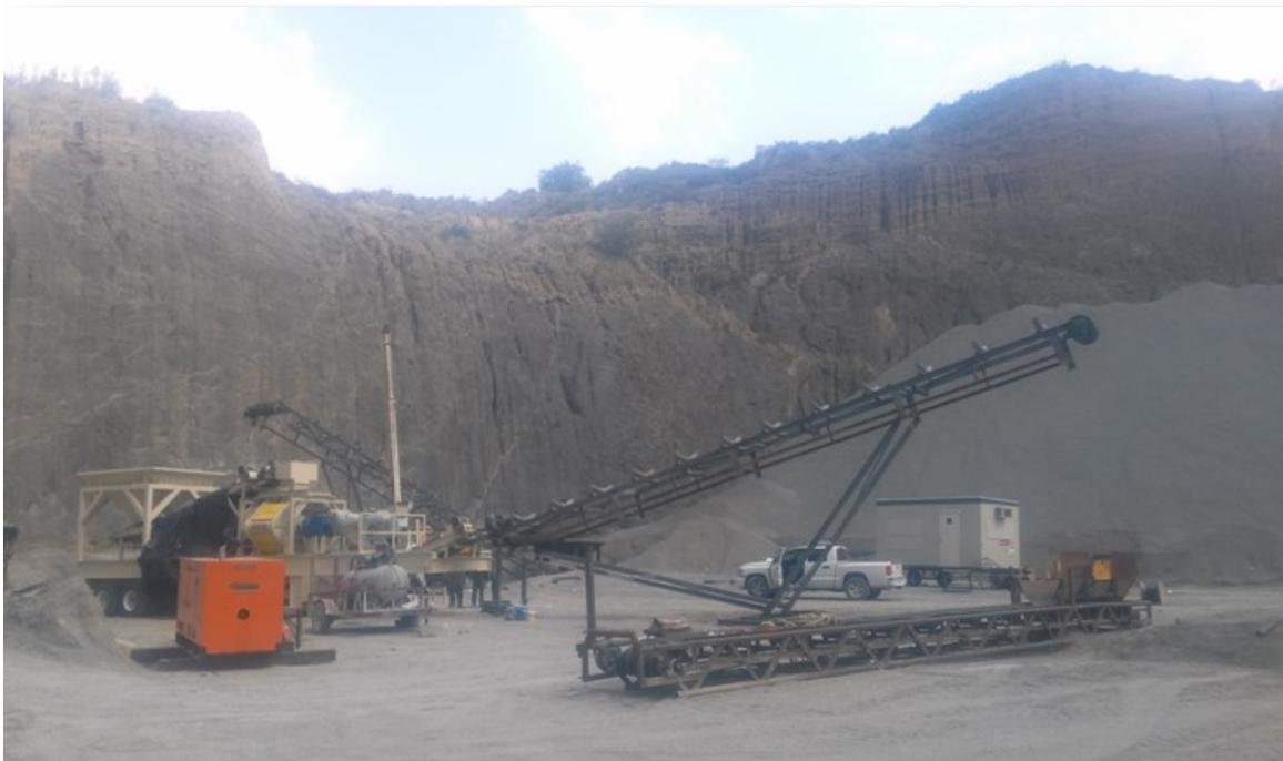
Figure 30: Metso portable High-pressure roller crusher.
