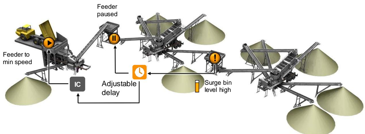
Figure 32: Functionality of a portable plant Intelligent Control, case tertiary crusher feed surge bin level high.
