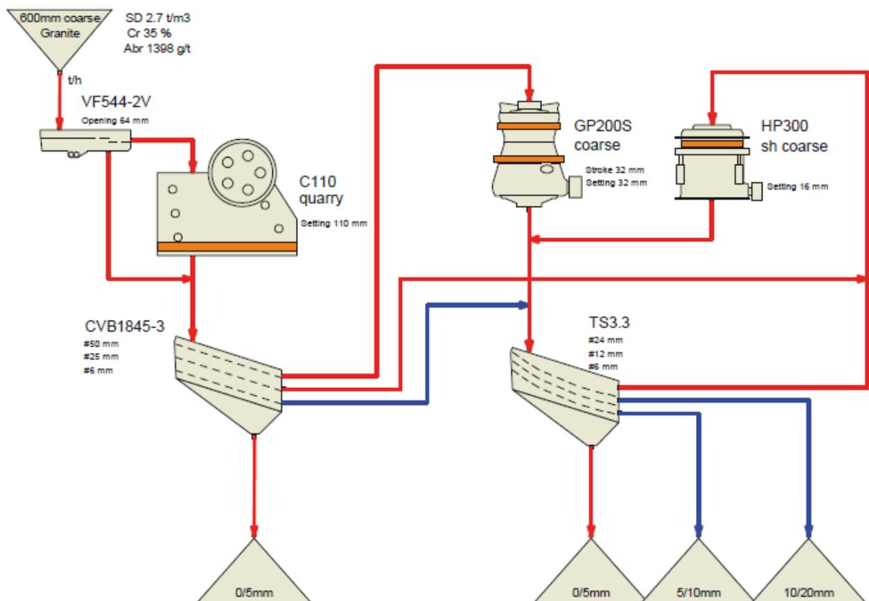
Figure 2: Process example 1: Three stage crushing plant, maximizing the capacity. All -20 mm particles screened directly into products. Capacity 320 tph.
