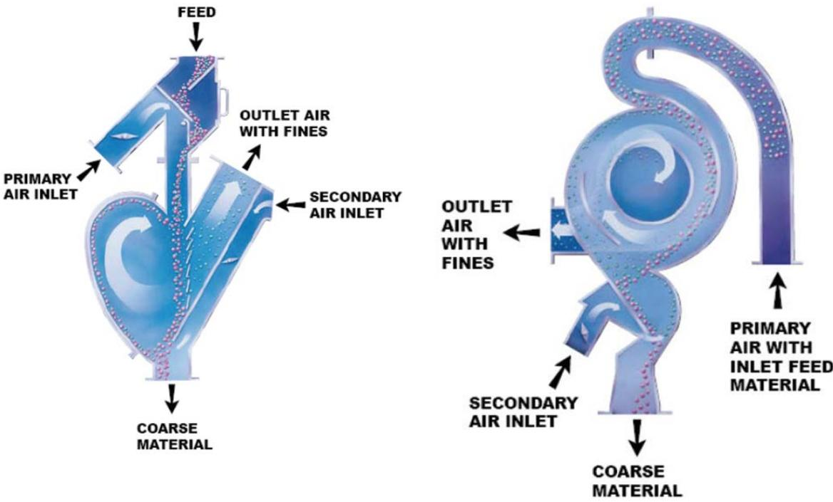
Figure 16: Metso static air classifier models Gravitational Inertial and Centrifugal.
