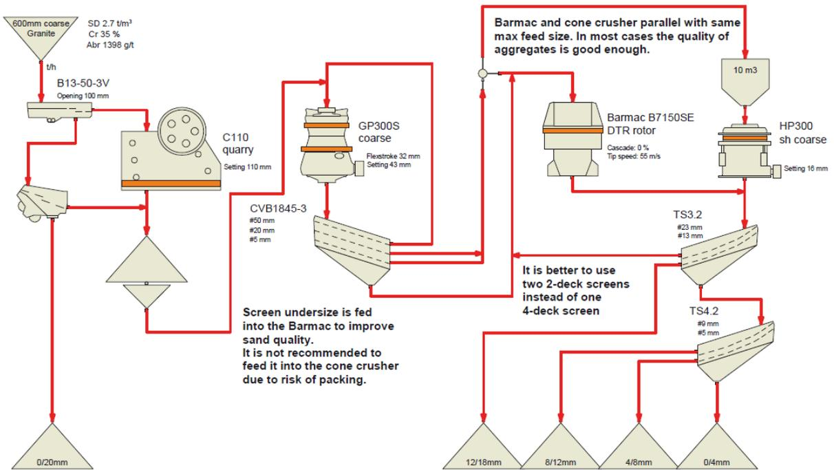
Figure 4: Process example 3: Concrete aggregates – 330 tph.
