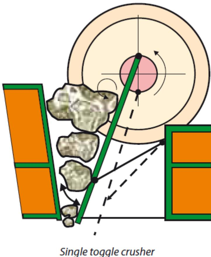
Figure 6: Single toggle crusher.
