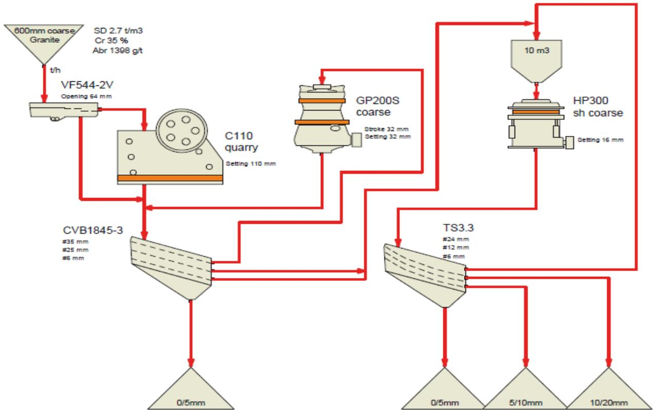
Figure 3: Process example 2: Three stage crushing plant, maximizing the quality. All products are done by tertiary cone. Capacity: 200 tph. Crushing equipment is same as in process example 1.
