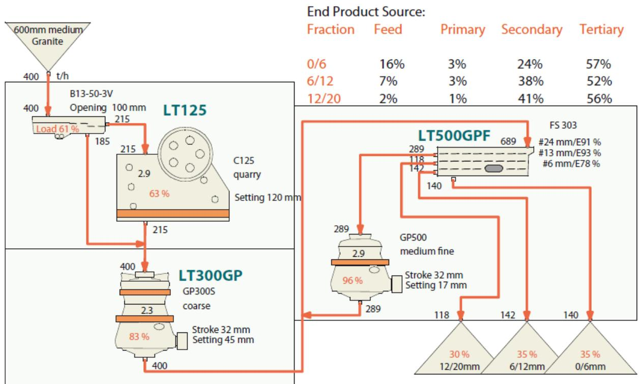
Figure 24: Asphalt aggregate production, lower quality or easy material.
