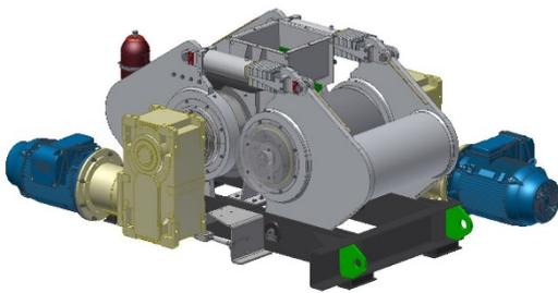
Figure 14: High pressure roll crusher.
