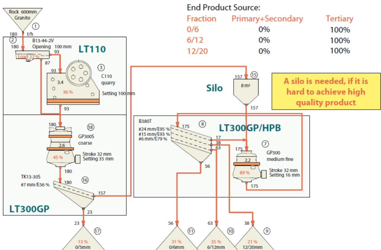
Figure 25: Asphalt aggregate production, high quality and/or difficult material.
