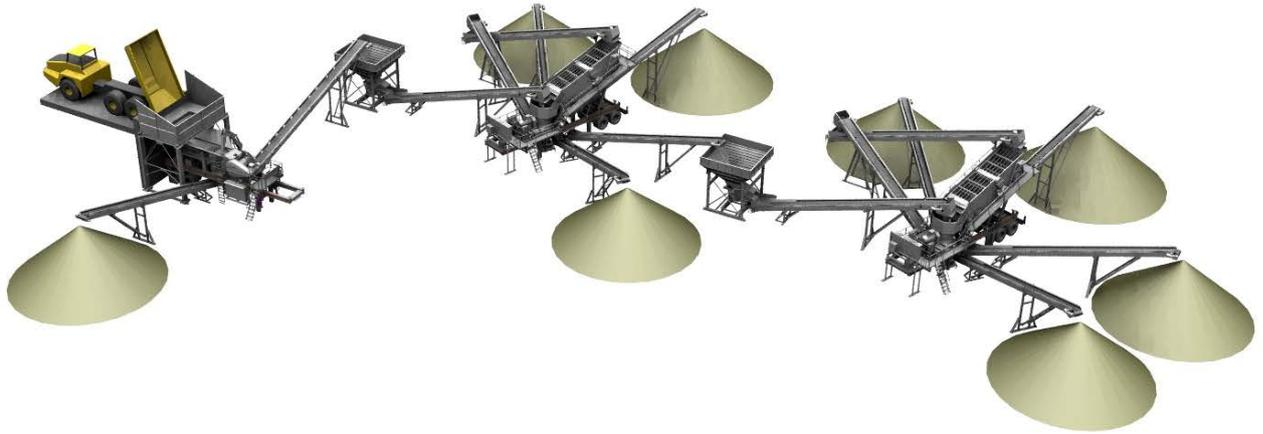
Figure 29: Portable crushing plant. Flowsheet possibilities.
