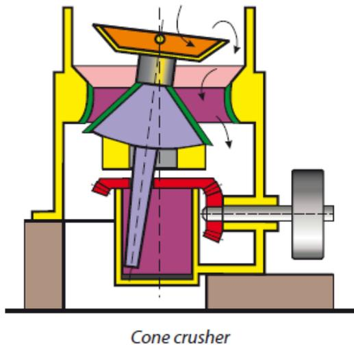
Figure 9: Cone crusher.
