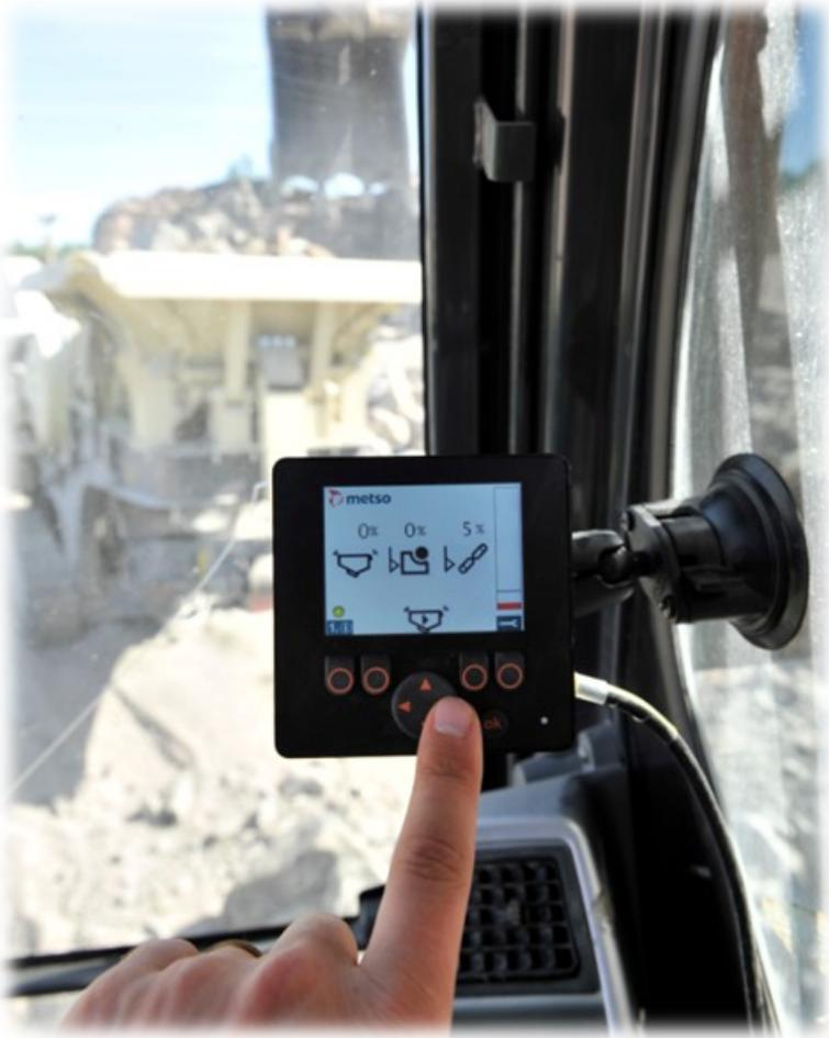
Figure 28: Crushing process control from excavator cabinet.
