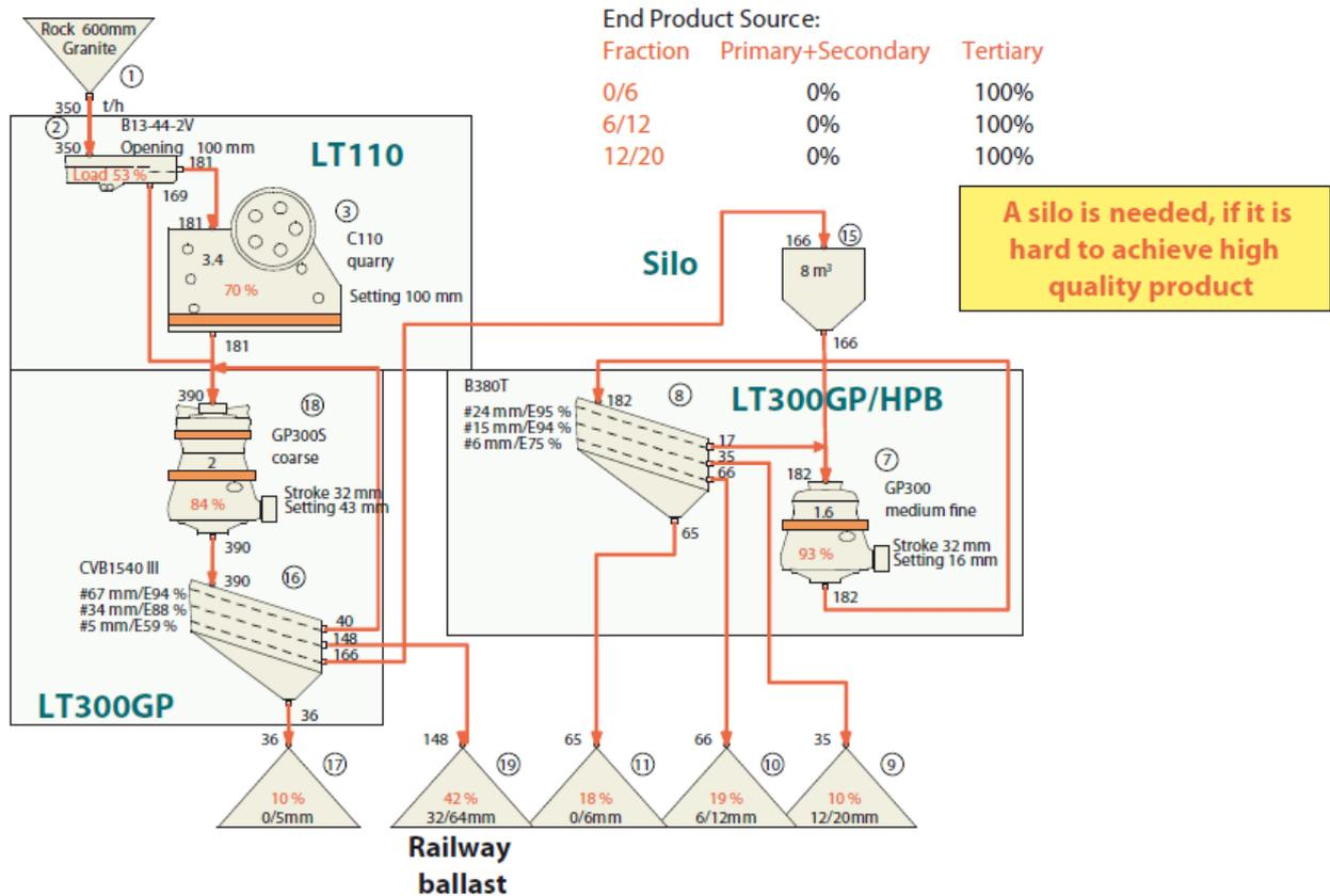
Figure 26: Combined railway ballast and high quality asphalt production.
