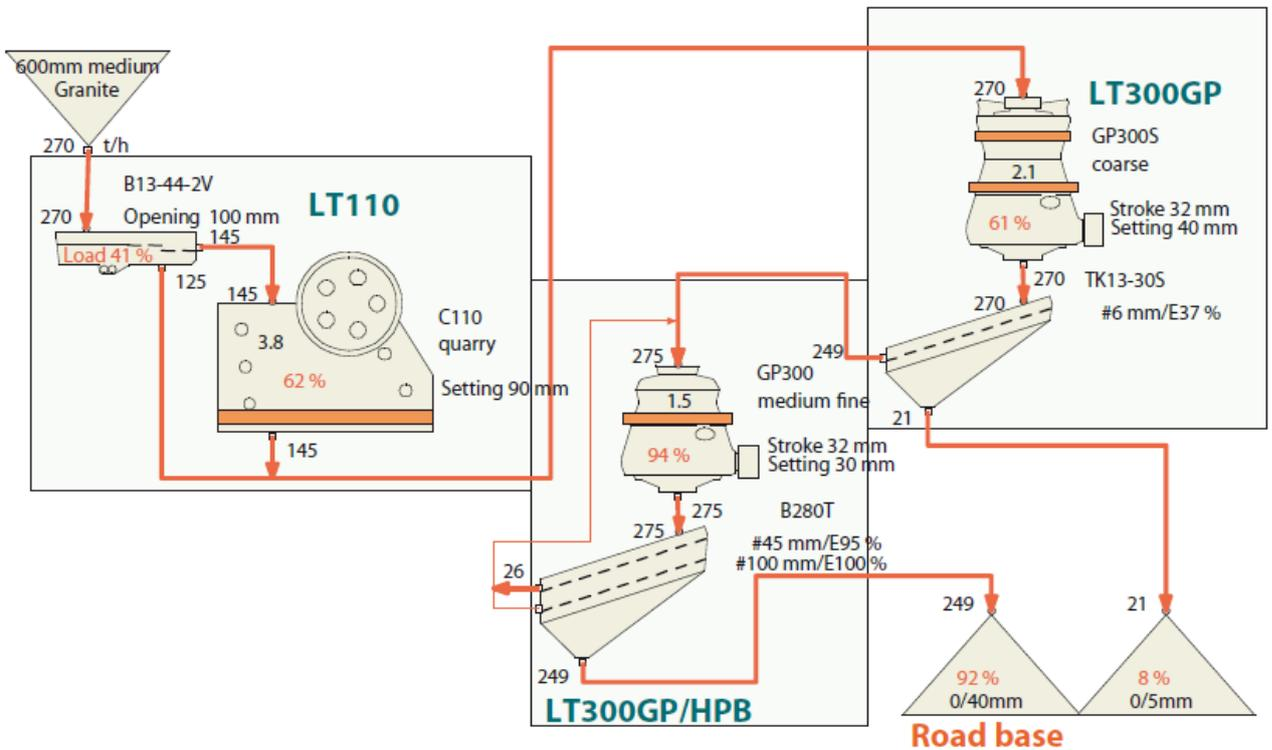
Figure 23: Typical road base production flowsheet when material is difficult.
