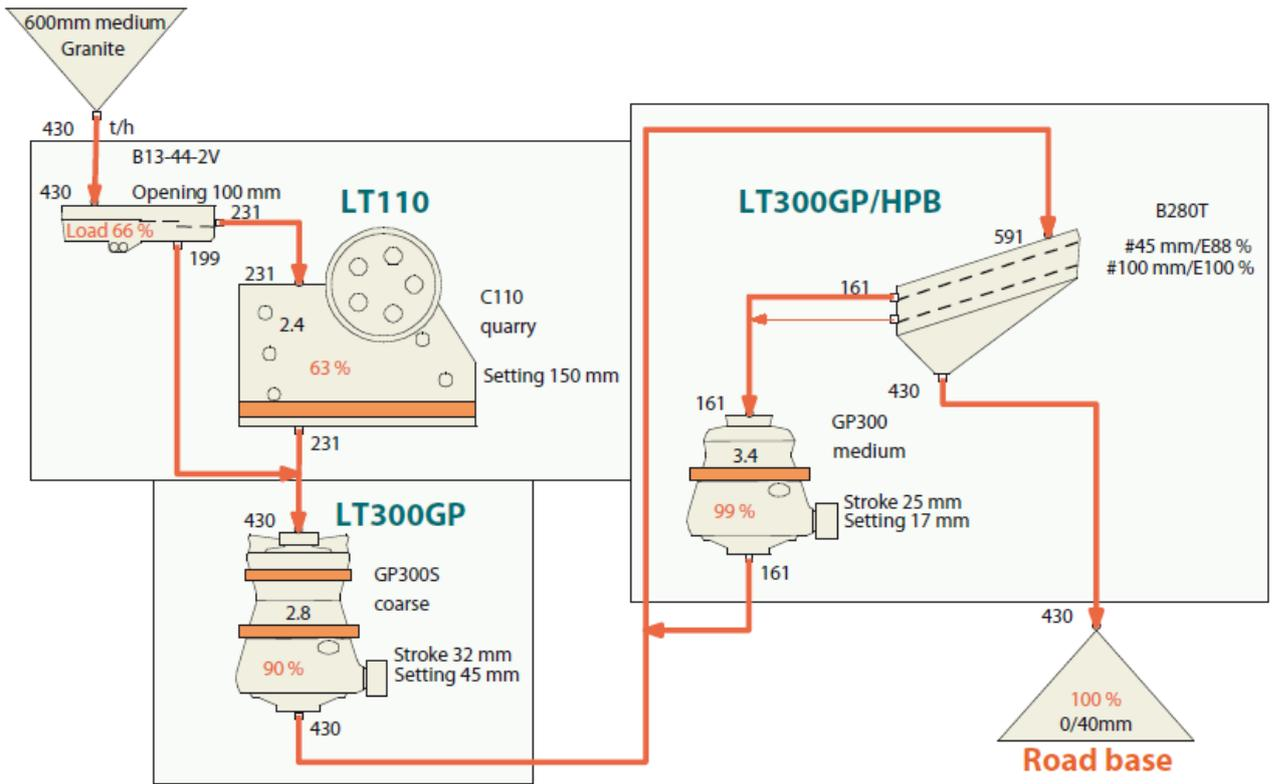
Figure 22: Typical road base production flowsheet when material is easy.
