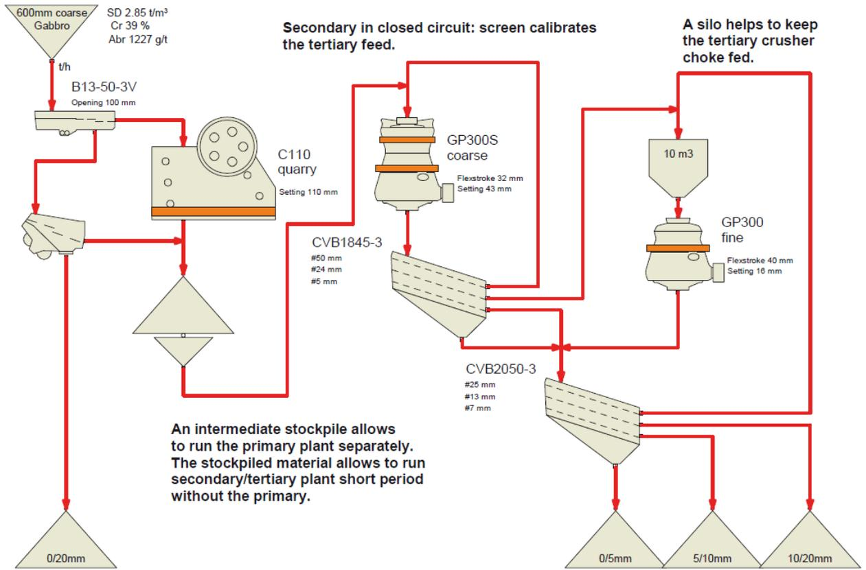
Figure 5: Process example 4: Asphalt aggregates – 330 tph.
