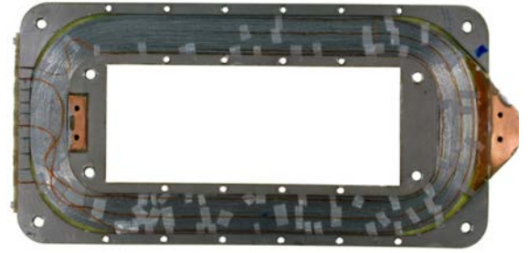
YBCO superconducting generator coil. (Courtesy DTU)
