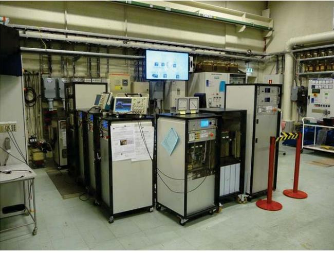
Laboratory testing of voltage droop control for a multi-terminal HVDC grid
