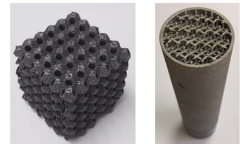
Figure 4. 3D printed metal foams as potential catalyst supports.
