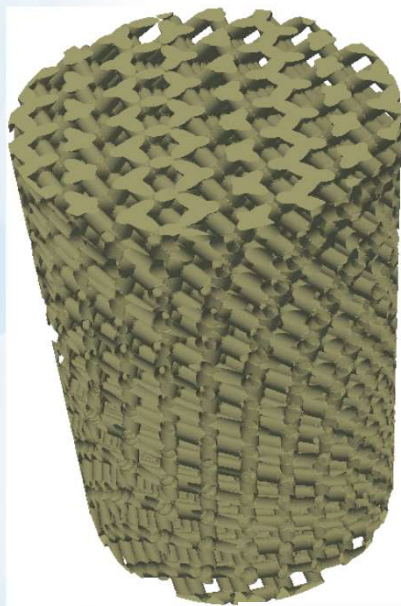
Foam structure (solid part)
