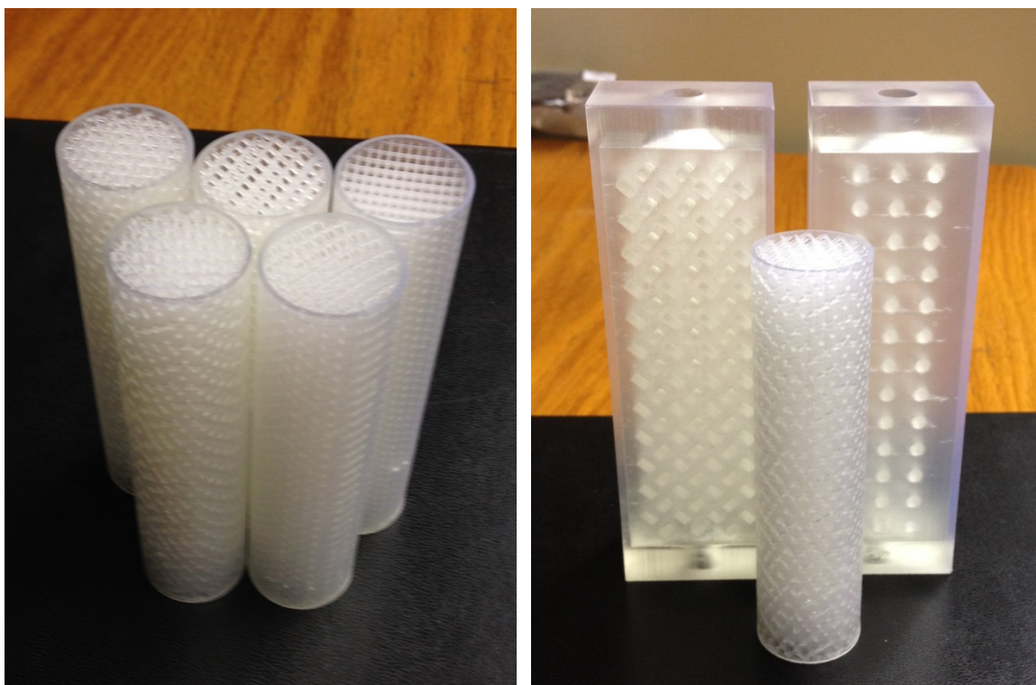
Figure 14 3D geometries manufactured with the SLA printer during the presentation to the 4 th year Chemical Engineering students.
