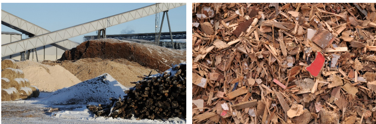
Fig. 3. Challenging fuels. 1) Snow covered fuels in winter (left), 2) chipped demolition wood (right)
