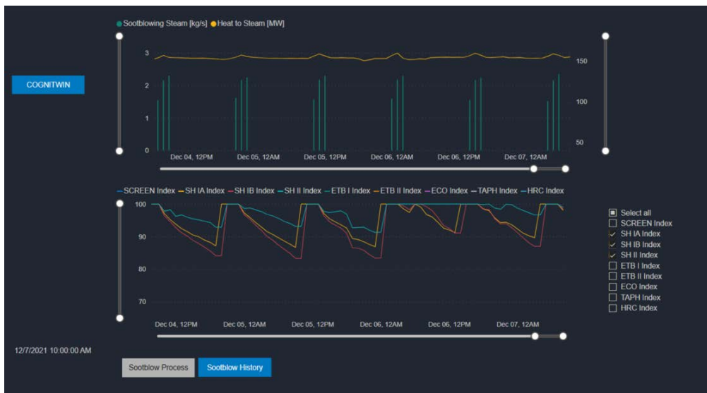
Fig. 20. Trend view of the COGNITWIN User Interface showing boiler load and sootblowing, and the heat transfer indexes describing the ability of each HX to transfer heat.
