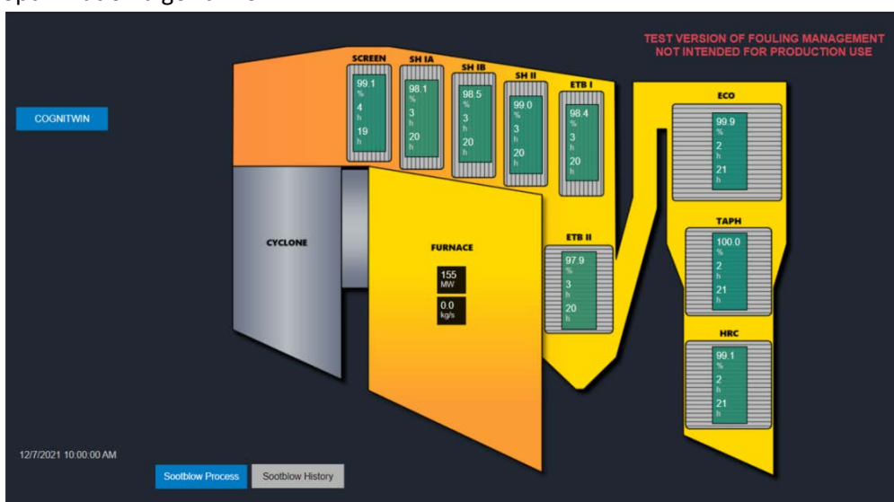
Fig. 19. User Interface of the COGNITWIN WP3 pilot showing the heat transfer indexes of heating surfaces.
