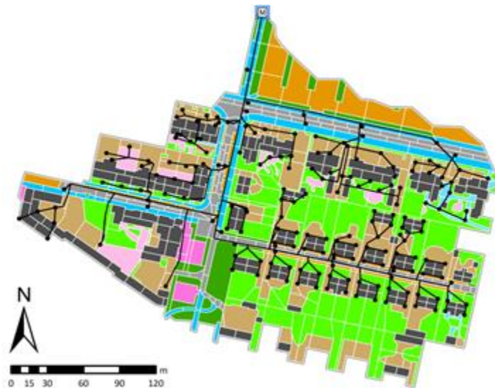
Figure 3: The high-resolution subcatchment delineation. Colours represent the surface subdivision based on different surface types, land-use types, and ownership classes; subcatchment boundaries are described with white lines, black lines represent the stormwater sewer network, and black dots indicate the sewer inlets (Krebs et al. 2014).
