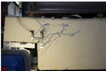
Prefabricated corbel end beams, Solution with fibres and alternative reinforcement configurations.
